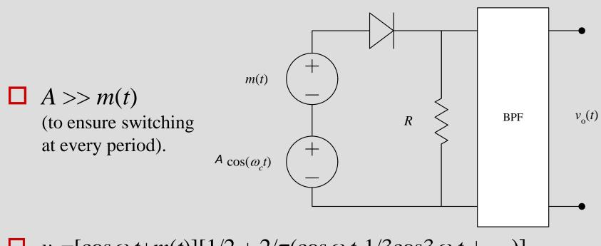
$v_R = [\cos \omega_c t + m(t)] [1/2 + 2/\pi (\cos \omega_c t - 1/3 \cos 3\omega_c t + ...)]$ = (1/2)  $\cos \omega_c t + (2/\pi)m(t) \cos \omega_c t$  + other terms (suppressed by BPF)  $v_o(t) = (1/2) \cos \omega_c t + (2/\pi)m(t) \cos \omega_c t$
