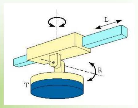
Consists of a sliding arm (L joint) actuated relative to the body, which can rotate about both a vertical axis (T joint) and horizontal axis (R joint)
