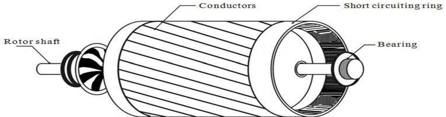
**Rotor of Squirrel Cage Induction Motor**
