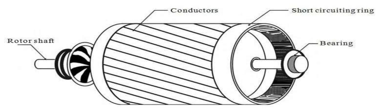
Rotor of Squirrel Cage Induction Motor
