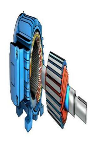
• The stator winding of a poly-phase I.M. is almost similar to the armature winding of a poly-phase alternator.
