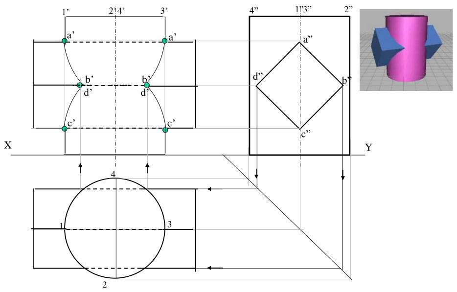
**Problem:** A cylinder of 80 mm diameter and 100 mm axis is completely penetrated by a cone of 80 mm diameter and 120 mm long axis horizontally.Both axes intersect & bisect each other. Draw projections showing curve of intersections.
