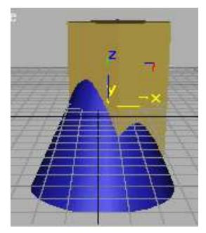
**Problem:** A cone70 mm base diameter and 90 mm axis is completely penetrated by a square prism from top with it's axis // to cone's axis and 5 mm away from it. a vertical plane containing both axes is parallel to Vp. Take all faces of sq.prism equally inclined to Vp. Base Side of prism is 0 mm and axis is 100 mm long. Draw projections showing curves of intersections.
