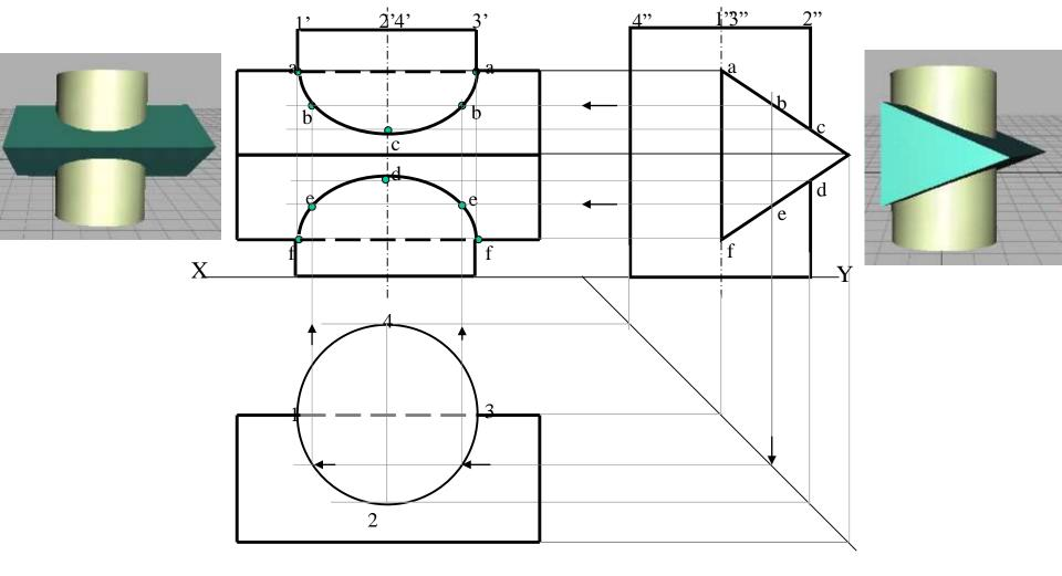
**Problem:** A sq.prism 30 mm base sides.and 70mm axis is completely penetrated by another square prism of 25 mm side s.and 70 mm axis, horizontally. Both axes Intersect & bisect each other.Two faces of penetrating prism are 30<sup>0</sup> inclined to Hp. Draw projections showing curves of intersections. CASE 6. SQ.PRISM STANDING & SQ.PRISM PENETRATING (30<sup>0</sup> SKEW POSITION)
