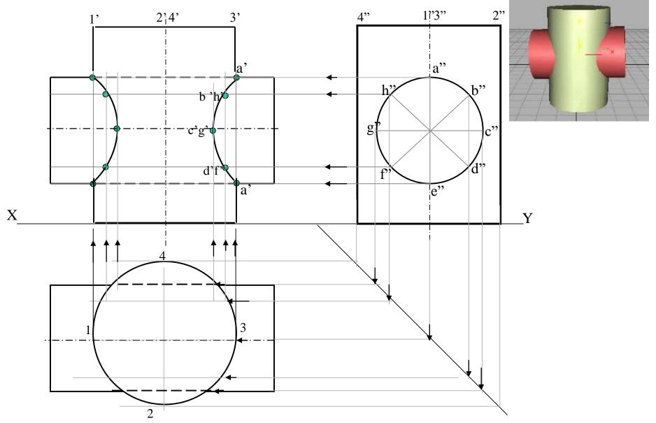
**Problem:** A cylinder 50mm dia.and 70mm axis is completely penetrated by a square prism of 25 mm sides.and 70 mm axis, horizontally. Both axes Intersect & bisect each other. All faces of prism are equally inclined to Hp. Draw projections showing curves of intersections.
